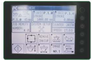
PLC touch screen control for easy printing parameter adjustment
